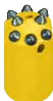
Model -33 All-round bit with six gauge buttons for medium hard to hard rock formations. Front and side flushing. Buttons inclined 15°.
